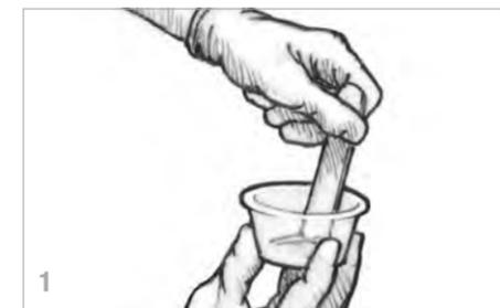
6. Dispense equal volumes of G/flex 650 resin and hardener into a mixing cup and stir thoroughly with the mixing stick (1). Transfer the mixed G/flex epoxy to the plastic syringe. (It is quicker to fill the syringe by removing the plunger and pouring the epoxy into top, especially in cooler temperatures. You should also find it easier to
