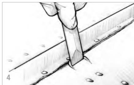
3. Keep forcing the mixture through the seam until you see epoxy on the other side of the hull. Thickened epoxy bridges gaps and stays in the seams while it cures.
