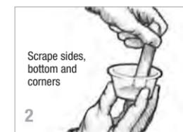
Resin and Hardener into a small mixing cup (1). Use a mixing stick to thoroughly blend the resin and hardener, while scraping the sides and bottom of the mixing cup (2). Small quantities can be mixed on a paper or plastic palette.
