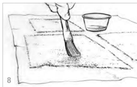
13. Place the three pieces of fiberglass on a piece of plastic. Using a disposable brush, apply the mixed epoxy to the pieces of fabric until they are saturated (8).
