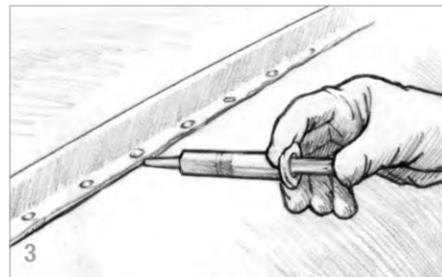
8. Apply a continuous bead of G/flex, using the syringe, along the heated seam and around rivet heads. The epoxy should thin out and flow into the smallest crevices (3). 9. Heat the metal with a torch or heat gun as necessary to thin the epoxy to a water-like consistency and to move it along and penetrate deeply into seams and under rivets. Continued moderate heating will cause the epoxy to gel and cure quickly. Do not heat the epoxy to the point where it discolors or begins to smoke.
