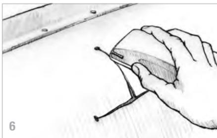
4. Abrade away any remaining paint in the area at least 2" larger than the hole on the inside and outside of the hull (6). (You can improve adhesion to aluminum by treating with an aluminum etch, such as the two-part WEST SYSTEM 860 Aluminum Etch. Follow the etch kit instructions.)
