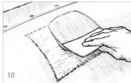
15. When both sides of the patch have cured to a duct tape-like tackiness, mix a batch of G/flex 650 and stir in enough 406 Adhesive Filler to thicken the mixture to a "mayonnaise" consistency. Using a plastic spreader, apply this mixture over the patch, filling and smoothing the uneven edges and blending both sides of the patch into the undamaged area around it (10). Allow the patch to cure overnight.
