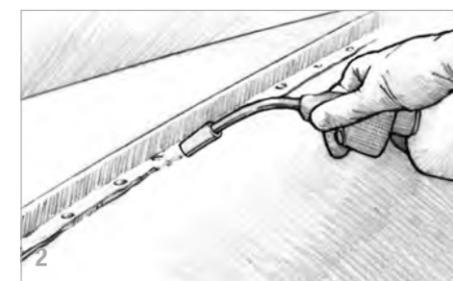
extrude the epoxy in cooler temperatures if you trim the syringe tip back to about a 1/16" opening.)
