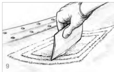
14. Position the largest piece of wet fiberglass over the hole on the inside of the hull with 2" of fabric extending beyond all sides
