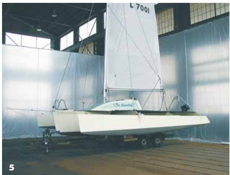
Figure 5—A completed L-7 trimaran. When folded, the L-7 is 8'4" wide and easily trailered.
