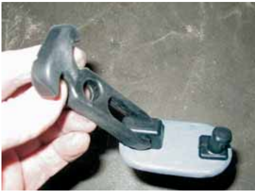
The latch and strike are mounted on a 1/4" plywood base plate (above). Blind fasten and bond them to the base plate using stainless steel flathead machine screws from the backside (below).
