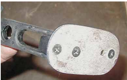
The latch and strike are mounted on a 1/4" plywood base plate (above). Blind fasten and bond them to the base plate using stainless steel flathead machine screws from the backside (below).
