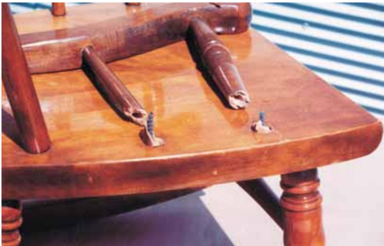
Above—The broken ends of the joints are drilled out and the cut off drywall screws are dry fit to assure the holes are aligned and deep enough.
