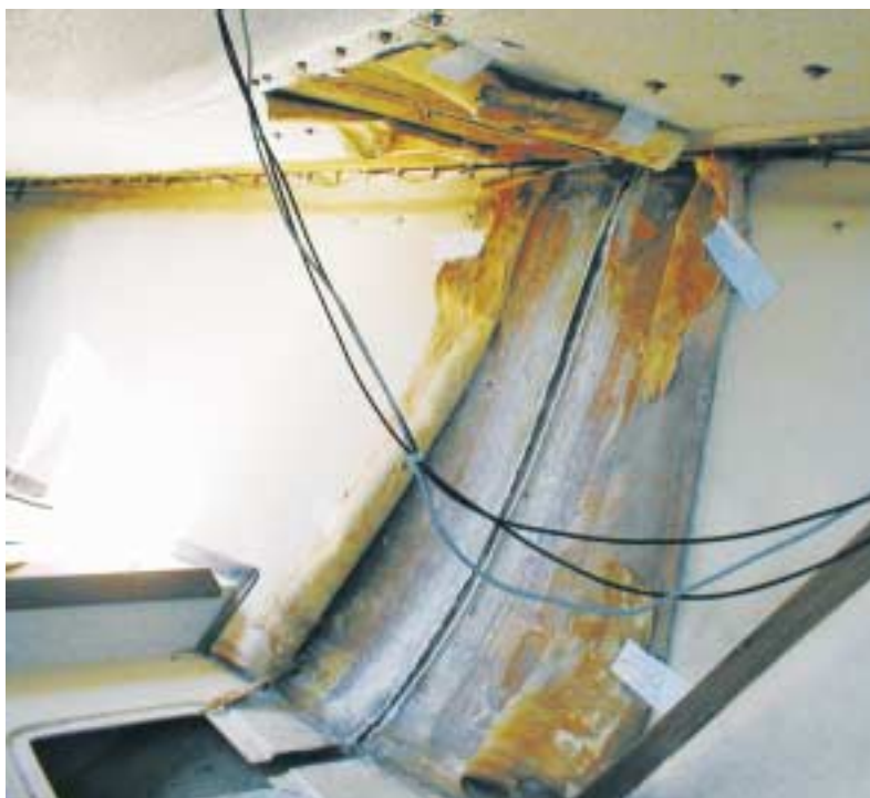
With the starboard bulkhead removed we were ready to remove the glass tabbing with a disc grinder.
