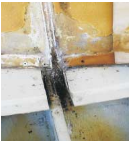
With the starboard bulkhead removed we were ready to remove the glass tabbing with a disc grinder.
