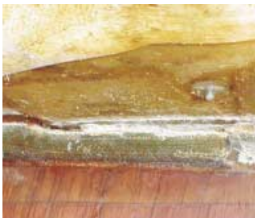
John used a Roto Zip to cut the tabbing where the bulkhead met the hull and deck. The Roto Zip cut quickly and raised minimal amount of dust.
