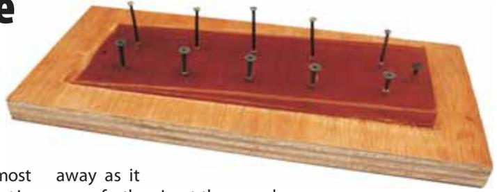
away as it cures further, I put the samples in an oven at 120°F for the weekend. I took the samples out and let them cool back down to room temperature. When I tried again, all was the same as before—no epoxy failures.
