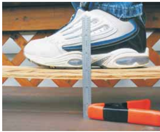
Left—An overview of the test apparatus showing the unreinforced board with no load applied.
