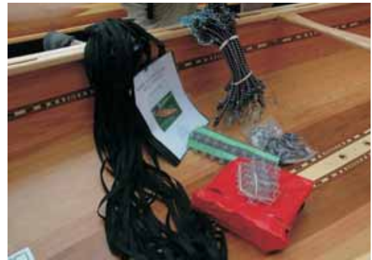
Above —The kit that allows you to clamp strips without the use of staples.
