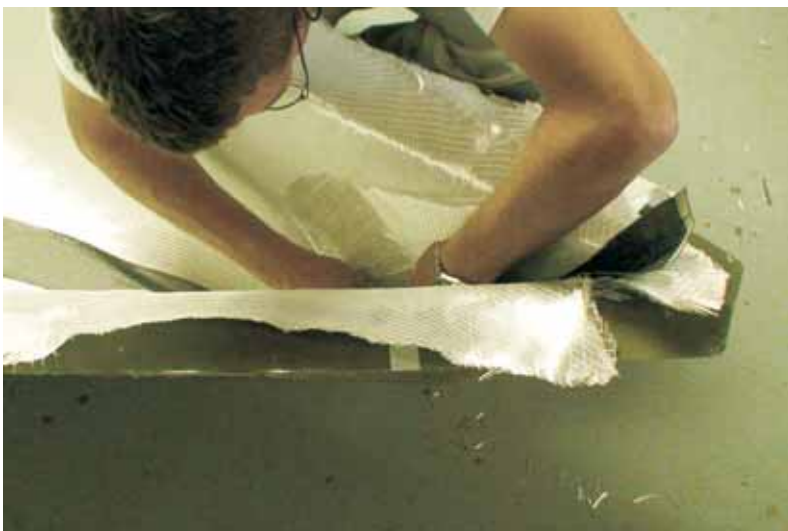
Alan Gurski installing layers of glass and carbon fiber tape into the mold for his resin infused version. He used two layers of 737 Biaxial Fabric, a thin foam core sandwiched between layers of 703 Unidirectional Carbon Tape followed by one more layer of 737.
