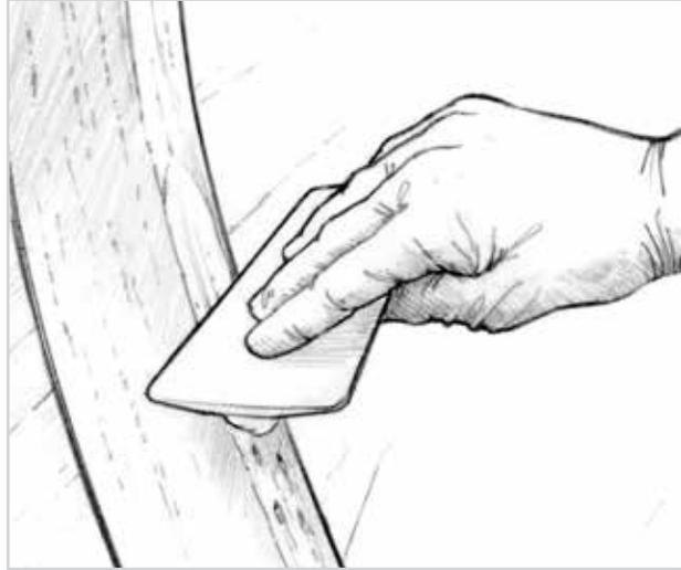
**Figure 3-5** Fill the remaining voids with fairing compound.
