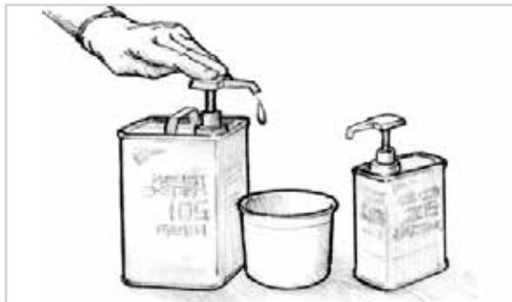
Figure 8-4 Dispense the proper proportions of resin and hardener.
