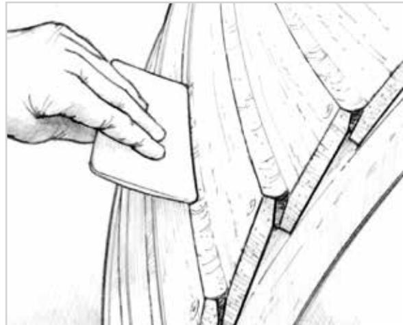
**Figure 5-9** Fill the wet-out seam with thickened epoxy.
