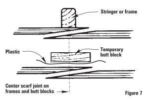
If the scarf joint does not land on a frame, you can still execute a strong scarf joint. Use a temporary butt block on the backside to receive the staples. Remember to put a layer of plastic under the butt block and tacking strips and prevent permanently gluing them to the plywood panels (See Figure 7).
