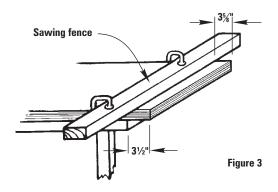
3. Select a straight piece of lumber at least a foot longer than your panel width to act as a sawing fence. The fence should be wide enough to resist bending in the center. A 4"-6" wide piece of ¾" plywood is adequate for a 4' cut, a 12"-16" wide fence for 8' cuts. Place it
