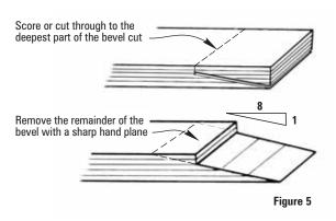
3. Position the panel on your bench so that the thin edge of scarf is fully supported. Using a sharp hand plane, remove the remainder of the wood between line marking the back edge of the bevel and the sawed
