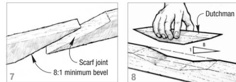
A DUTCHMAN is a wood splice used to repair damaged sections of wood timbers. We recommend creating an 8:1 bevel (8) on each end of the joint to provide adequate gluing area to maintain structural integrity.
