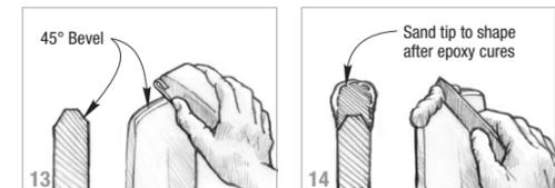
Mix an appropriate amount of G/flex 650 thickened with 406 Colloidal Silica Filler to a mayonnaise consistency. Apply a thick bead of the thickened mixture around the edge of the paddle blade (14). Apply additional thickened epoxy to extend the tip, if desired, after the initial application has gelled and will support the additional weight.
