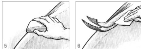
Apply a coat of epoxy to the sanded/treated area. Lay the largest piece of fiberglass onto the wet epoxy. Apply more epoxy to wet out the fiberglass cloth. If necessary, a heat gun can be used to warm the epoxy and improve wet out on heavier fiberglass fabrics. Use a spreader to smooth the fabric and remove excess epoxy (6).
