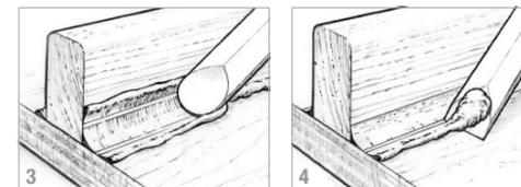
onnaise consistency, along the inside corner of the joint. Form the epoxy into a cove section using the round end of a mixing stick (3). Clean off the excess epoxy with the beveled end of the mixing stick before the epoxy gels (4).
