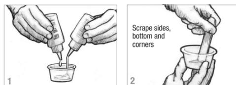
After mixing the resin and hardener, you will have about 45 minutes, at 72°F (22°C), to apply the mixture before it begins to gel and up to 75 minutes to assemble and clamp parts after the epoxy is initially applied. At 72°F (22°C), the epoxy mixture will solidify in 3–4 hours and reach a workable cure in 7–10 hours—the epoxy may be sanded, clamps can be removed, and joints can be moderately loaded. Wait 24 hours before subjecting joints to high loads.
