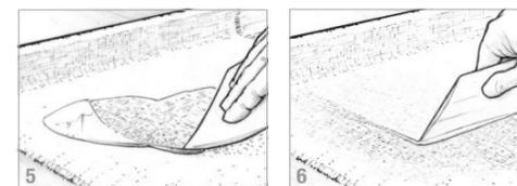
Coat the substrate with epoxy. Lay the fabric in position on the wet epoxy. Spread mixed epoxy onto the fabric using a plastic spreader (5). When the fabric and substrate have been saturated, use the spreader to smooth and remove excess epoxy (6). Repeat the process with additional layers.
