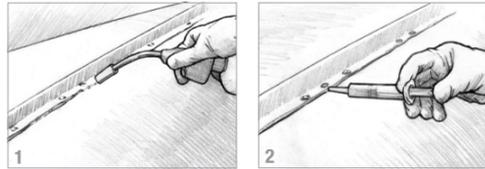
Inject the epoxy with the syringe or apply it with a small brush along the seam while the metal is still warm (2). The epoxy will thin when it touches the warm metal and will flow deep into the crack. Use the heat gun to warm the metal along the seam as you direct the epoxy into it. The heat will help release air in the epoxy and speed the cure.
