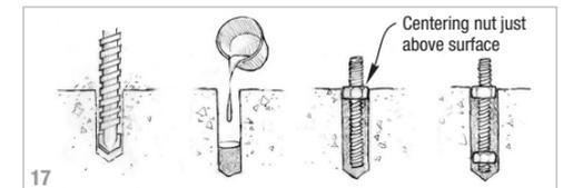
It's a good idea to put a nut on the threaded rod so that its top is barely above the surface (17). This centers the rod in the hole and will help to reduce the creep load on the epoxy when the hardware item is tightened down. ■
