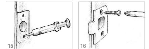
The easiest method is to simply wet out new pilot holes (or stripped fastener holes) (15) with G/flex 650 prior to installing the screws (16). The epoxy will soak into the exposed end grain on the inside of the hole, effectively increasing fastener diameter. This results in more holding power, and seals water out so the wood stays drier and stronger.
