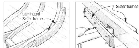
LAMINATING multiple layers of wood strips is a great way to create custom-shaped lumber for frames, sister frames, legs, arches, railings, and trim. Laminated lumber is stronger and more stable than steambent or sawn lumber. Glue strips using the preparation and bonding techniques on the reverse page. Use a jig or mold to clamp strips to the desired shape (11, 12). Jigs should be strong enough to provide even clamping pressure and prevent springback until the epoxy cures. ■
