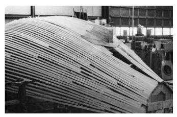
**Figure 20-6** A ribband mold for an IOR ½ ton racer. Note the use of shorter ribbands to fill gaps between full-length ribbands. The skeg shown was laminated out of veneers beforehand, then secured to the mold. The veneer used to plank the hull was bonded to the skeg. This was done to save the extra expense and time of molding such an extreme shape during general laminating.
