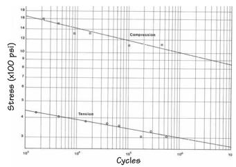
Figure C-13 Tangential Fatigue.
