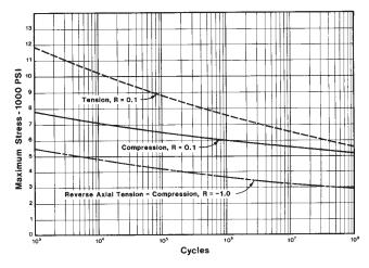
**Figure 3-3** Laminate fatigue properties. Maximum strength adjusted to 12% wood moisture content vs. total cycles for BG-1 Douglas fir/epoxy laminate with 12:1 slope scarf joints with 3" stagger, 31.8 in<sup>3</sup> test volume, parallel to grain load direction, at room temperature.
