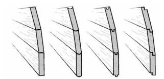
**Figure 23-1** Four common strip edge profiles: (1) square edged (2) bead and cove, (3) tongue and groove and (4) ship lap.
