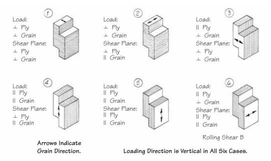
Figure C-15 Various Shear Loading Possibilities for Blade Laminate.
