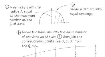
On the deck beam stock lay out the true  $\mathfrak{D}$  width of the deck (half is shown for clarity). Erect the camber height A as a perpendicular at the  $\mathfrak{C}$ . Then mark each half of the baseline, from the centerline to sheer, into the same number of sections as (2). At these sections mark off the corresponding dimensions B, C, D perpendicular to the baseline. Finely fair a batten through your marks on both sides of the  $\mathfrak{C}$  to obtain your deck camber curve.
