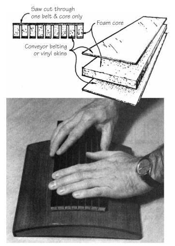
**Figure 23-18** Custom sanding blocks can be made by bonding flexible belting material to a wood or foam core. Vary the core thickness and the saw cut spacing to adjust the flexibility for various curved surfaces.
