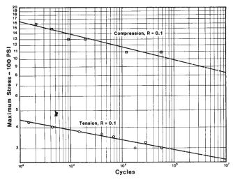
Figure 3-6 Tangential fatigue, wood/epoxy laminate.
