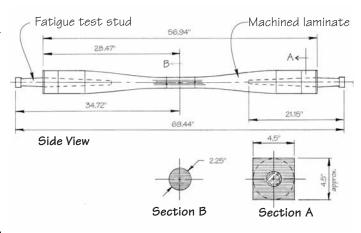
Figure C-7 Detail of "dogbone" type fatigue test specimen.
