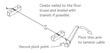
**Figure 16-5** An arrangement for tightening the baseline cable.
