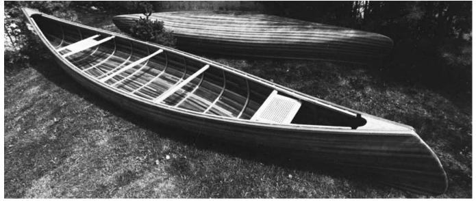
**Figure 23-12** Two stripper canoes built by Herschel Payne. Western red cedar and WEST SYSTEM epoxy were used for both boats. The 15' (4.5m) model weights 32 lb (12.8kg) and the 18' (5.5m) model weighs 48 lb (21.6kg).
