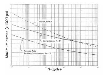
Figure C-10 Primary fatigue properties of wood.
