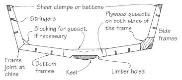
**Figure 24-1** Typical frame assembly showing gussets, filler blocking, and the position of structural members.
