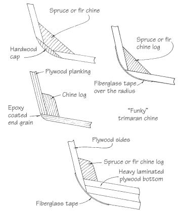
Figure 24-4 Details of typical chine joints.
