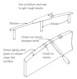
Figure 18-9 Beveling mold frames.
