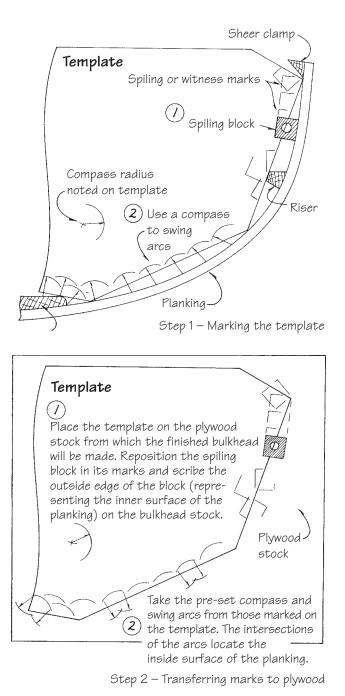
**Figure 26-11** Two methods for transferring the hull shape to a template and then to plywood.
