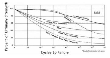
Figure C-1 Tensile Fatigue Comparison.
