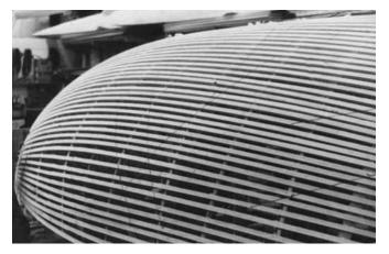
**Figure 21-2** A ribband mold for a ½-ton racer showing alignment markings for various veneer layers.
