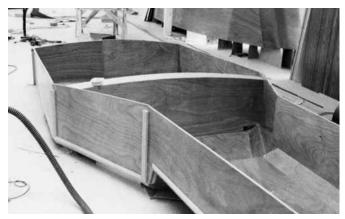
Figure 27-12 A cockpit assembly constructed outside the hull.
