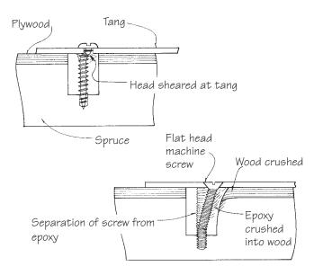
**Figure 14-6** Cross section view of failure modes for shear on self-tapping screws and flathead machine screws.
