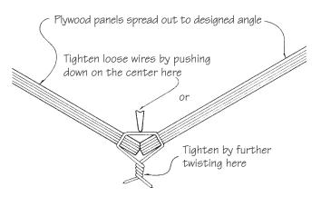
Figure 25-8 Tightening wires at the keel joint.
