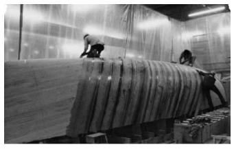
**Figure 23-8** Laminating the first layer of veneer over faired planking. Note the planking bench to the right.
