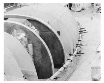
**Figure 19-11** Laminating a sheer clamp over the outside of mold frames. No notches have yet been cut in the molds. When it has cured, the sheer clamp is removed, dressed and prefinished. Then it is fit to notches in the molds.
