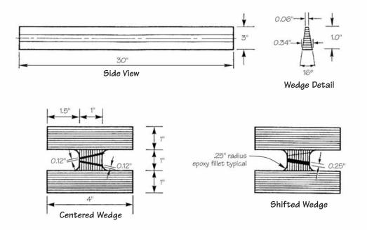
Figure C-11 Longitudinal wedge joint test specimen details.
