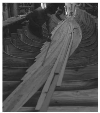
**Figure 23-14** Planking being installed on a mold for the hull of the Formula 40 trimaran *Adrenalin*. The hull was built in left and right female molds rather than the typical male hull and deck molds.
