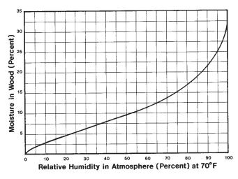
Figure 3-11 Equilibrium moisture content as a function of relative humidity.
