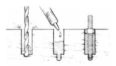
**Figure A-20** Bond threaded rods or studs into the substrate as an alternative for easily removable hardware.
