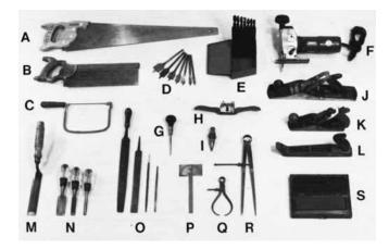
Figure 8-2 Broader small tool inventory: (A) crosscut saw;
