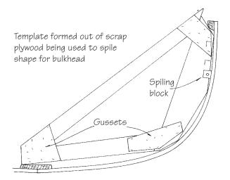
**Figure 26-10** A template built up with scrap lumber and plywood gussets.
