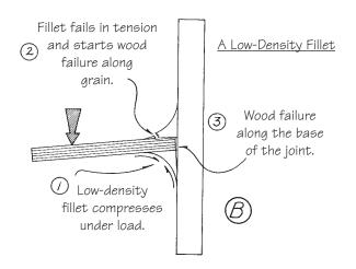
**Figure 11-18** Failure mode for proper sized fillet radius is shown in Cross Section A. Failure mode for inadequate sized fillets is shown in Cross Section B. The chart shows the radius size required for high-density fillets to produce a wood failure (A) rather than a joint bond failure (B). Results vary depending on plywood quality and thickness, and filler density. Experiment to find the proper radius for the materials you are using.
