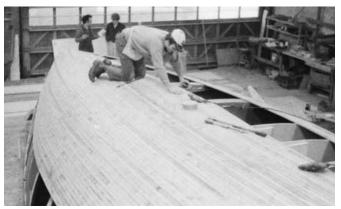
**Figure 23-4** Strip planking a 42' (12.8m) hull. These strips are being laid from a master plank from the bilge up to the keel.
