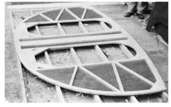
**Figure 26-12** A major structural bulkhead for *Golden Dazy* is constructed with a framework sandwiched between two  $\frac{1}{2}$ " (12mm) thick panels of utile plywood.
