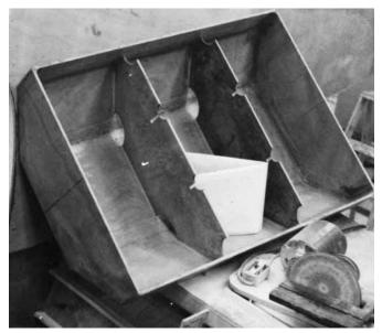
**Figure 26-23** A 40-gallon (150 liter) tank for *Rogue Wave*, constructed using fillets and fiberglass tape on all inside joints. The top of this tank forms a part of the cabin sole and the tank is removable. Baffles are scalloped on the upper edge so each compartment will vent. Notches at the bottom of the scallops are for  $\frac{3}{6}$ " (9mm) thick longitudinal plywood frames to support the top.
