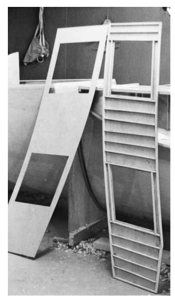
**Figure 11-15** Cockpit seats showing an inner skin bonded to the framing and a matching outer skin. Core material can be cut to fit the spaces within the frames. In this case the framing itself was adequate to support the plywood panels.
