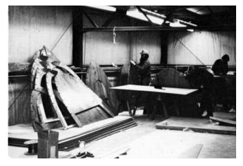
**Figure 17-9** Prefinishing permanent frames for a 60' (18m) trimaran.
