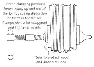
**Figure 11-7** Uneven clamping pressure forces epoxy out of the joint, causing distortion or a twist in the timber. Clamps should be placed in the middle of the laminate, spaced evenly and tightened with consistent pressure.
