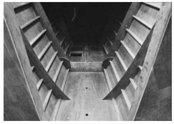
Figure 26-20 The forepeak cabin sole with lift-out sections.
