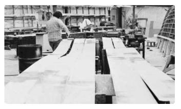
Figure 22-13 Coating 40'  $\times$  1' (1200mm  $\times$  2400mm) panels of planking stock. Scarfing together long lengths of planking stock like these cuts down on scrap rate.
