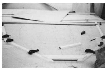
**Figure 17-4** Fitting and assembling frames for a double chine trimaran hull on lofted sections.
