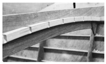
Figure 27-8 Triangular notches were cut into a laminated beam before it was bonded to the plywood frame. Longitudinal deck stringers were then easy to fit into the notches.
