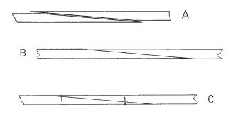
**Figure 12-3** When bonding thin stock or more than one scarf, take care to avoid overmatching the bevels (A) or undermatching the bevels (B). Use wire brads or staples to hold a bevel in proper alignment (C) and prevent slipping during clamping.
