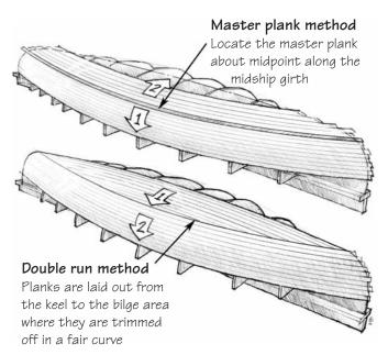
Figure 23-2 Two methods for strip planking hulls.
