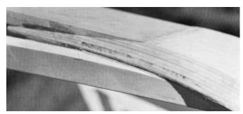
**Figure 19-4** A laminated stem scarfed to a solid keel. Note the stringer bonded to the stem.
