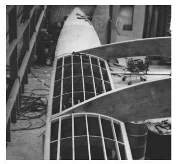
Figure 27-2 The same deck beams with stringers in place, ready for decking.
