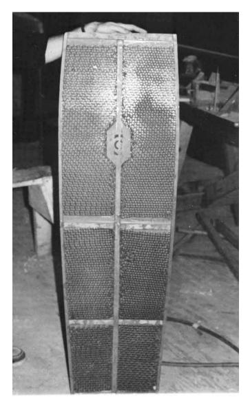
**Figure 11-10** A DN-class iceboat hull bottom showing honeycomb core material between frames. The outer plywood skin has not yet been bonded to this panel.
