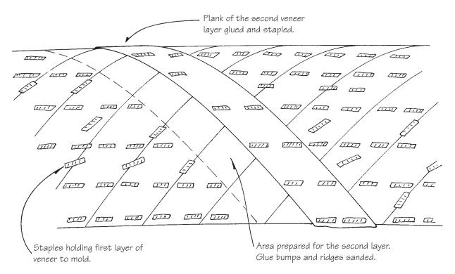
**Figure 21-19** Marking and preparing a hull for the second layer of veneer. Note that staples are left in the first layer until planks of the second layer are spiled.
