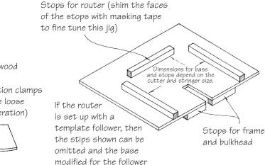
Figure 22-3 A router jig for notching frames and deck beams prior to set-up.
