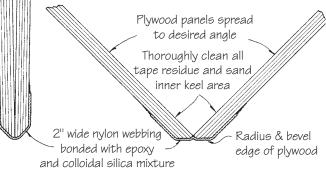
Figure 25-4 Joining plywood hull panels with nylon webbing.
