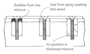
Figure 14-11 Potential problems with bonded fasteners.
