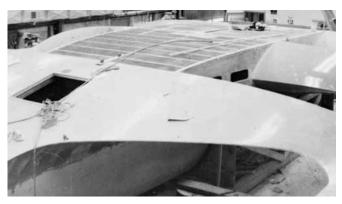
**Figure 27-17** The foredeck and beam fairings on *Rogue Wave* are plywood over stringers. The cabin areas are sandwich construction using resin-coated paper honeycomb core.
