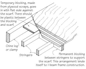
**Figure 24-9** Blocking between stringers for scarfing plywood in place.
