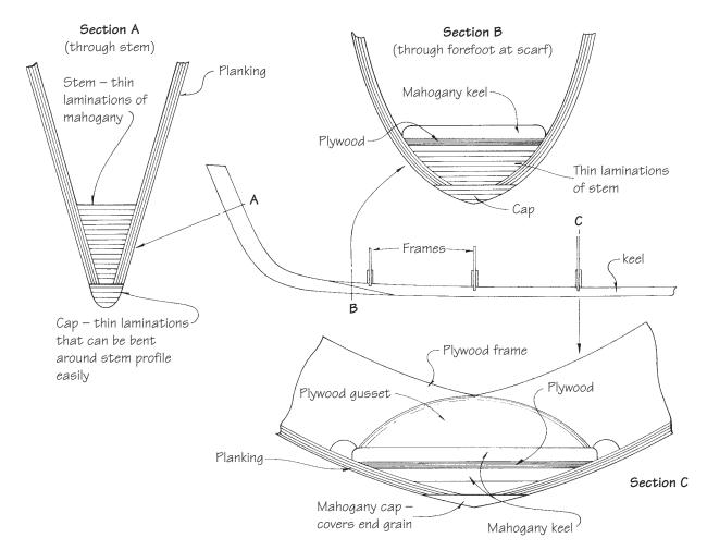
**Figure 19-1** Three section views through the stem and keel of the 60' (18m) trimaran *Rogue Wave*. Note the plywood laminated into the main keel. The cross-grain in this lamination counteracts the splitting forces of the keel or centerboard.
