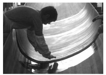
**Figure 23-16** Applying unidirectional carbon fiber to the inside of the right half of *Adrenalin's* hull. The two halves were joined after the interior was finished and a bulkhead was installed.
