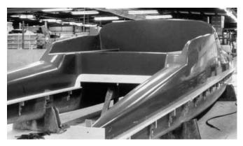
**Figure 20-2** A plug for a 32' (9.7m) catamaran is polished and waxed, ready for a mold to be cast. The mold for the upper surface will be female in the areas of the hulls and cabin top and male in the cockpit area.
