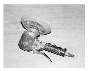
**Figure 8-8** A 7" electric orbital polisher is used with a foam disc pad for sanding.
