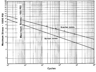
**Figure 3-5** Tension fatigue. Maximum stress vs. total cycles for Douglas fir/epoxy laminate with 12:1 slope scarf and butt joints with 3" stagger, 31.8 in<sup>3</sup> test volume, parallel to grain direction, room temperature and 12% wood moisture content.
