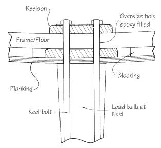
Figure 14-19 Cross section view of bonded keel bolts.
