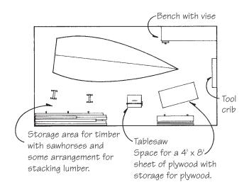
**Figure 8-12** Layout for a typical home shop for building a 25' to 30' (7m-9m) boat.
