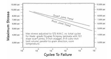
**Figure C-9** S-N diagram. Tension fatigue test showing scarf joint and butt joint trend lines. (R=0.1)
