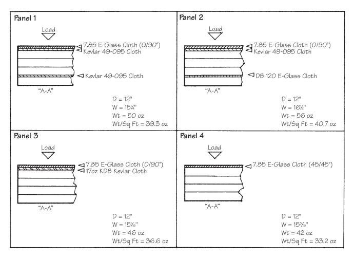
Figure E-1 Test samples constructed of synthetic fibers, cedar, and WEST SYSTEM® epoxy. Arrow indicates direction of impact load.
