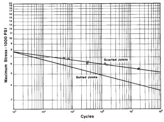
**Figure 3-4** Compression fatigue. Maximum stress vs. total cycles for Douglas fir/epoxy laminate with 12:1 slope scarf and butt joints with 3" stagger, 31.8 in<sup>3</sup> test volume, parallel to grain direction, room temperature and 12% wood moisture content.
