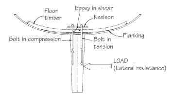
**Figure 14-20** Cross section view demonstrating design considerations in bonded keel bolts. Tension and compression forces are transmitted as a shear load by the resin bond between the keel bolt and the wooden structural members. Bonded keel bolts are immobilized and there is no chance for the edge of the ballast keel to crush the soft planking of the hull bottom. Bonding also keeps the keel bolt nuts and washers from embedding into the keelson.
