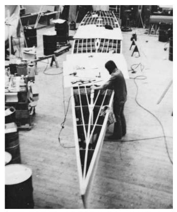
**Figure 27-19** Fitting and scarfing the  $\frac{3}{16}$ " (5mm) plywood deck on the main hull of the proa *Slingshot*. Note the pads and blocking for hardware that are fit between stringers and frames.
