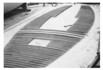
**Figure 27-21** Scrap strips of plywood are used as core framing for a sandwich deck.
