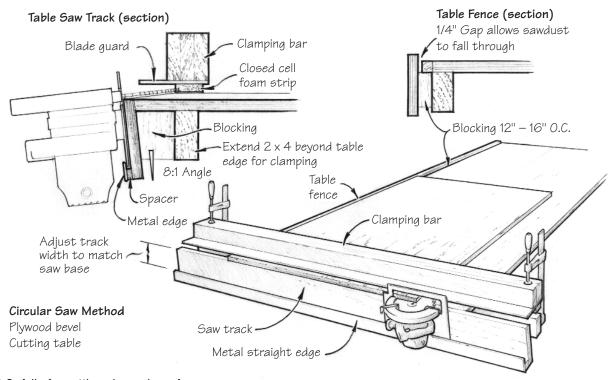
Figure 12-9 A jig for cutting plywood scarfs.
