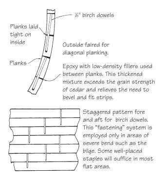
Figure 23-6 Doweling to prevent plank misalignment.
