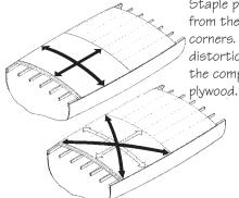
Staple plywood deck panels from the center out to the corners. This will minimize distortion and rippling from the compounding of the plywood.
