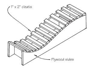
Figure 11-3 A simple form for laminating wider pieces.
