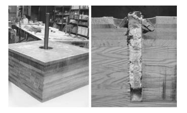
**Figure 14-4** The  $1^{1}/2^{"}$  test samples before testing (left) and a cutaway of the damage after testing (right). The  $1^{1}/2^{"}$  silicon bronze threaded rods were imbedded perpendicular to the glue joints.
