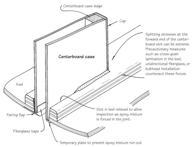
Figure 19-10 Detail of a centerboard case construction and installation.
