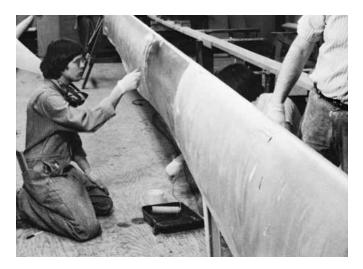
**Figure 13-4** Wetting out the fiberglass cloth on a wing mast for the 60' proa *Slingshot*. In this application, 4 oz cloth was draped over the spar and wet out with rollers.
