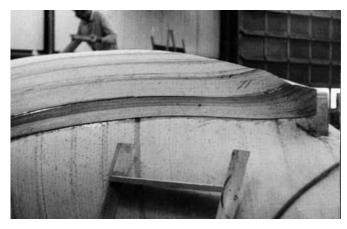
**Figure 21-5** More staples are necessary to hold down thin veneers in a reverse or concave area near a skeg. Note the reasonably regular stapling patterns employed on planking in the foreground.
