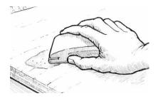
**Figure A-23** Sand cured fairing compound to the desired contour.
