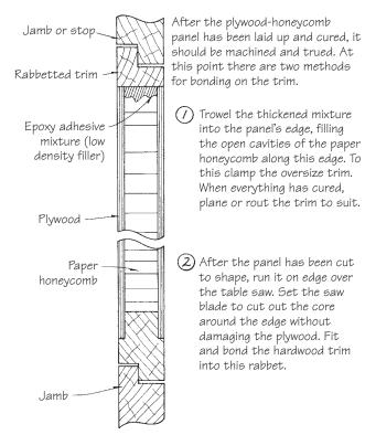
**Figure 26-15** A section though a door showing the honeycomb core and skins with two methods of bonding trim to the panel.
