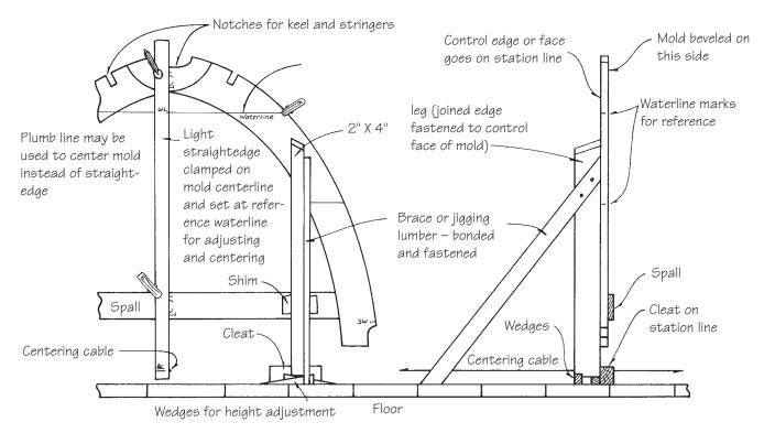
Figure 18-5 Two views of a typical frame set.
