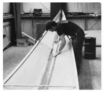
**Figure 25-10** Applying glass tape over a keel fillet on a 30' (9.1m) hull.
