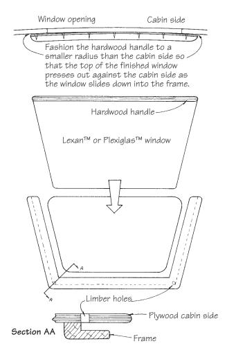
Figure 26-26 Low-cost lift-out window.
