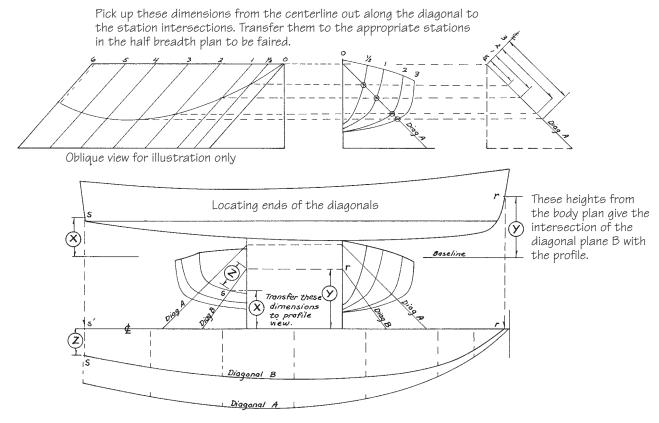
Figure 16-9 Laying off diagonals.
