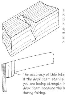
This method of notching for deck beams uses the high shear strength of the epoxy to advantage while maintaining the integrity of the carling or sheer clamp.
