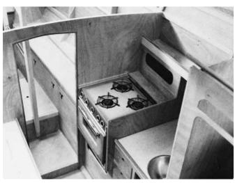
**Figure 26-16** A galley in a 30' (9.1m) trimaran with a bulkhead forward and a hanging locker at lower right.
