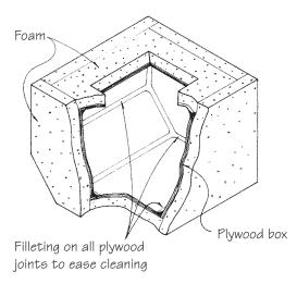
Figure 26-21 Cutaway of inner icebox construction.
