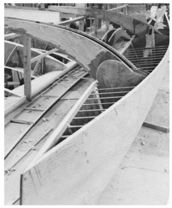
**Figure 25-26** Tension flanges for deck I-beams are bonded to the underside of the sheer clamp. Sheer webs for deck I-beams will be bonded to the top of these flanges. They will look like the deck beams in Figure 25-24.
