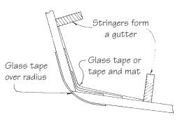
**Figure 24-12** A taped composite chine with conventional stingers.
