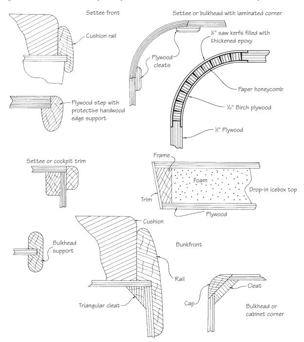
**Figure 26-9** Design details for interior joinery. The basic designs are universal to boatbuilding, but modifications can be made to lighten the structures without sacrificing strength because they are bonded. We usually use fillets and triangular cleats instead of square stock for interior construction and get the same bonding area for less weight. It's easy to form corner pieces for settees, bulkheads, and other molded items over common objects such as pipes and barrels.
