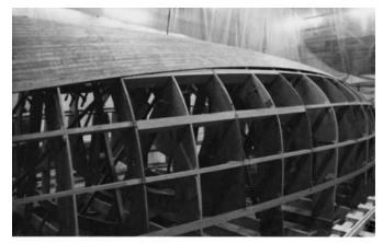
Figure 23-3 Strip planking a mold.
