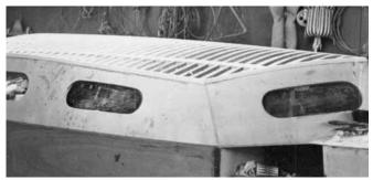
**Figure 27-26** A cabin roof built over a cabin top and temporary forms inside the cabin. Small,  $\frac{1}{2}$ " wide  $\times \frac{3}{4}$ " thick (12mm  $\times$  18mm) ribs spaced on 4" (100mm) centers were laminated over the interior ply and faired smooth. Blocking for a headsail track was inserted at the edge of the cabin and a  $\frac{3}{16}$ " (5mm) plywood roof was laminated over the assembly.
