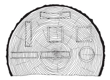
**Figure 3-9** Shrinkage and distortion for wood of various cross sections as affected by the direction of annual rings. Tangential shrinkage is about twice as great as radial. (From *Wood as an Engineering Material*, U.S. Department of Agriculture Handbook, No. 72, p. 3-10.)
