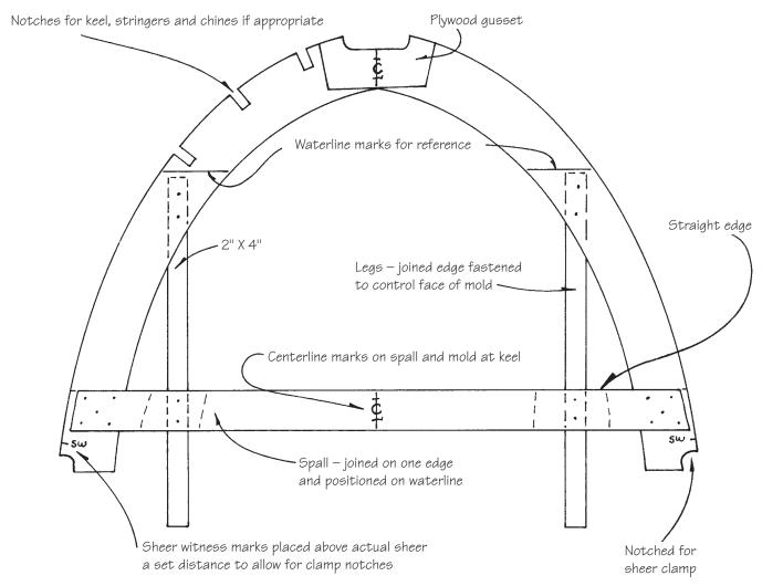
Figure 17-5 A typical mold frame with legs and spall installed and reference lines marked.
