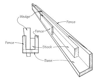
Figure 12-1 Basic scarfing jig.
