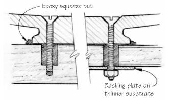
**Figure 14-15** Tighten fasteners or increase clamping pressure until a small amount of epoxy squeezes from the joint.
