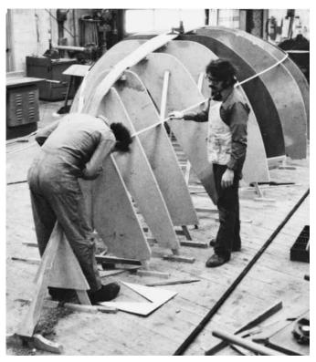
**Figure 19-5** The keel/stem assembly is fit to molds for the 32' (9.7m) *Hot Flash.* Molds are notched so the keel lies flush with the control face of the mold. Note the blocking used to secure the keel/stem assembly to the molds.
