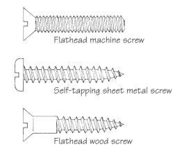
Figure 14-2 Typical screw types.
