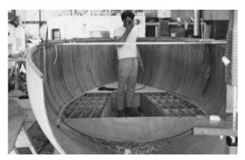
**Figure 26-6** The transom is left open for easy access to the interior. Structural bunks are also airtight buoyancy tanks for this lightweight laminated sloop.
