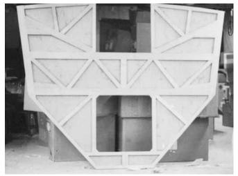
**Figure 24-2** Load-bearing bulkheads can be made from two pieces of thinner plywood with a framework sandwiched in between. The bulkhead arrangement shown above handles the main beam loads from a trimaran's outriggers.
