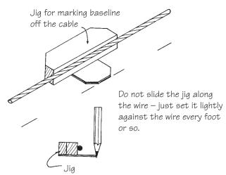
**Figure 16-6** A jig or gauge for transferring the baseline to the lofting board.
