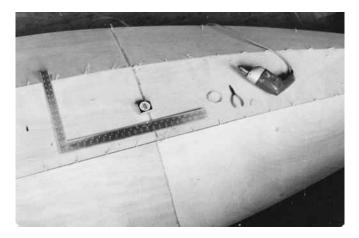
**Figure 24-13** Panel joints of a Fireball dinghy temporarily held with wire. Fiberglass tape will be laid on the inside of these joints and the wires will be removed. After fairing, fiberglass tape or cloth will be will be applied to the exterior of the joints. (Photo by Mark Lindsay)
