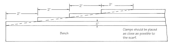
**Figure 12-12** Stacking <sup>1</sup>/<sub>4</sub>" thick panels to cut several 8-to-1 scarf bevels simultaneously. The setback of each panel is based on the panel thickness and bevel ratio.
