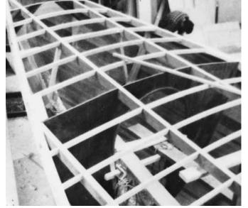
**Figure 27-5** Longitudinal and smaller athwartship beams on *Golden Dazy*.
