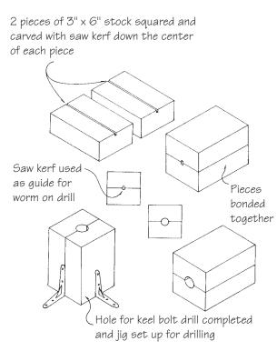
Figure 14-22 A jig for drilling keel bolt holes.
