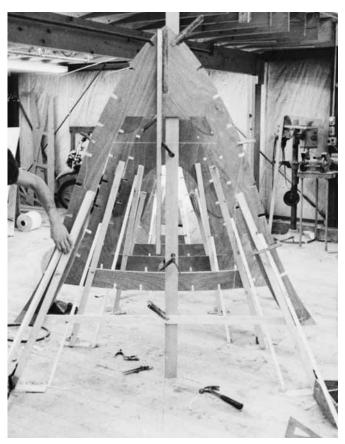
**Figure 18-8** Setting up frames. Note the wedges on the floor under the legs. The frame in the foreground is clamped to its anchoring block and the diagonal bracing. A straightedge is clamped along the frame's centerline and just touches the centerline cable at floor level.
