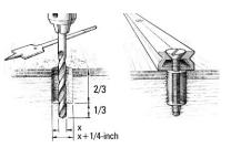
**Figure A-16** Drill oversized holes to increase the exposed substrate area and the amount of epoxy around the fastener.
