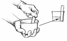
**Figure A-3** Stir resin and hardener together thoroughly—at least one minute, longer in cooler temperatures.
