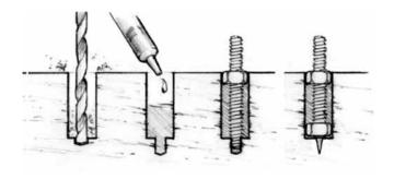
**Figure 14-9** Bond threaded rods or studs into the substrate as an alternative to bolts or screws for easily removable hardware. This is a useful variation for engine, motor, or machine installations. You can eliminate the pilot hole by adding another nut to the bottom of the threaded rod for alignment.
