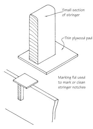
Figure 22-5 A marking gauge or fid.
