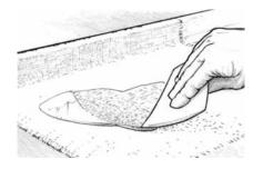
**Figure A-24** Spread epoxy over the cloth surface with a plastic spreader.
