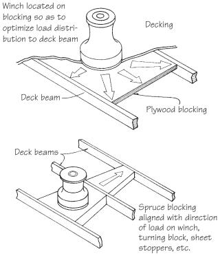
Figure 27-22 Hardware blocking details.
