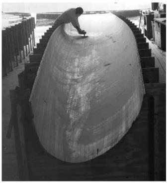
**Figure 23-15** Fairing the inside of the right half of *Adrenalin's* hull after the cedar planking is installed.
