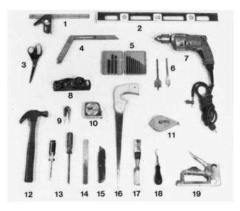
**Figure 8-1** Minimal small tool inventory: (1) combination square; (2) 24-inch level; (3) scissors; (4) sliding bevel or bevel square; (5) basic drill bit assortment; (6) spade drill bits as needed; (7) electric drill motor; (8) block plane; (9) compass; (10) 25-foot tape measure; (11) chalk line; (12) hammer; (13) screwdrivers; (14) rasp; (15) utility knife; (16) keyhole saw; (17) chisel; (18) staple removing tool; (19) staple gun.
