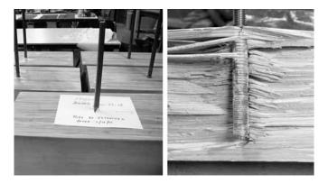
**Figure 14-3** The  $\frac{3}{4}$ " test samples before testing (left) and a cutaway of the damage after testing (right). Threaded rods were imbedded parallel to the glue joints.
