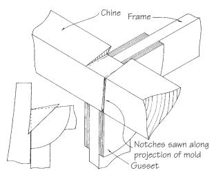
Figure 24-5 Notching the chine at the frame.
