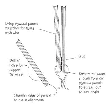
Figure 25-5 Joining plywood hull panels with wire.
