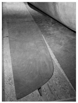
**Figure 25-2** Plywood panels for a Tornado catamaran. These panels are cut from 5mm okoume plywood.
