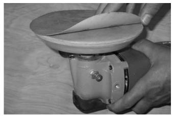
**Figure 8-6** A foam disc pad used with the 7" electric orbital polisher. We bond a piece of  $\mathcal{H}_{6}$ " birch plywood (or plastic laminate) onto the face of the disc. The plywood is flexible enough to follow major contours, yet is effective for sanding and fairing uneven surfaces with varying densities, such as cured epoxy with various fillers.
