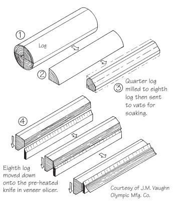
Figure 9-2 Manufacturing sequence in veneer slicing.
