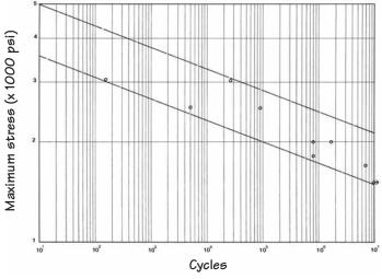
Figure C-3 Torsional Shear Fatigue.
