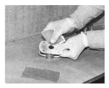
**Figure 14-12** Sand the bonding surface of steel and bronze fittings with coarse sandpaper.
