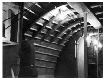
**Figure 26-4** Interior construction in an upside-down hull of an IOR ½ ton racer. Lighting and tools are set up in the hull. Note the band saw in the background at the far right.
