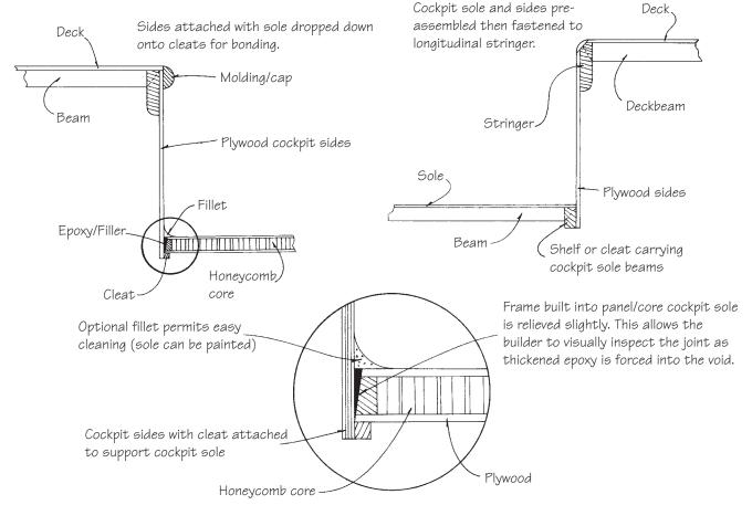
Figure 27-16 Cockpit construction details.
