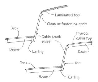
Figure 27-27 Construction details for cabin sides and tops.
