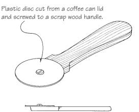
This tool was recommended to us and it does a good job. The plastic discs can be made to any radius and are easy to clean.
