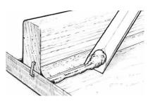
Figure A-14 Clean up the excess epoxy outside of the fillet margin.
