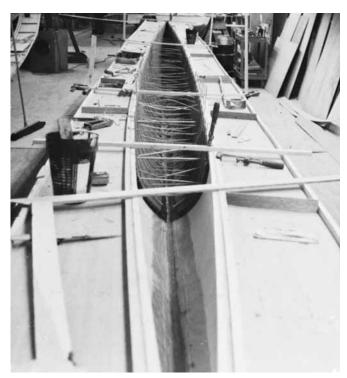
**Figure 25-18** Bonding resin-coated paper honeycomb panels to the inside of a folded plywood hull. Sticks are providing clamping pressure by forcing the honeycomb against both sides of the hull. When this laminate has cured, 12 oz fiberglass cloth was bonded to the interior side of the honeycomb core.
