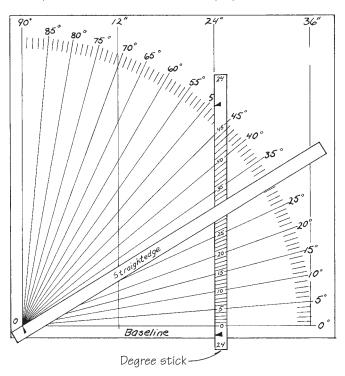
Mark the degrees using the straightedge over the bevel board. Be sure to note the proper control edge and station spacing.
