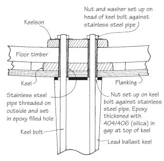
Figure 14-26 Cross section of a removable bonded keel.
