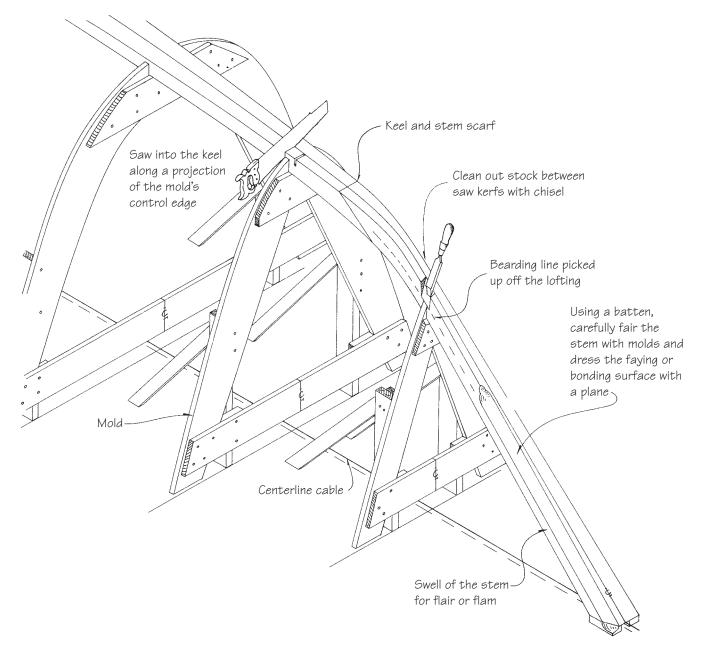
**Figure 19-7** A set-up for a typical IOR racer. Control lines have been drawn on the stem. Notches are cut in the keel at the molds to determine bevels. The stem is blocked up to allow the centerline cable to pass freely underneath.
