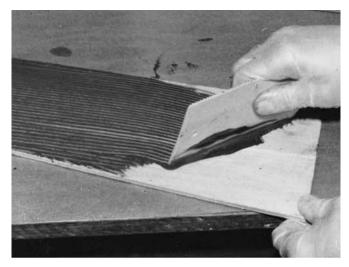
**Figure 11-13** Applying thickened epoxy with a modified plastic spreader. Cut notches in the edge, sized and spaced to suit the desired rate of application.
