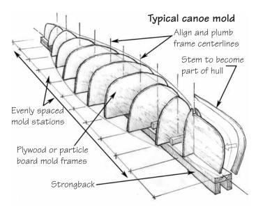
Figure 23-17 A typical canoe mold with plywood frames.
