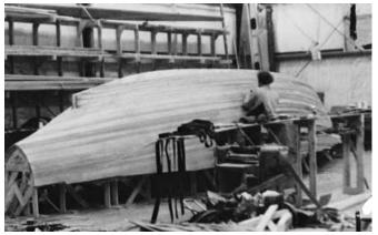
Figure 21-22 The final layer of veneer is laid fore and aft on this IOR  $\frac{1}{2}$ -ton racer.
