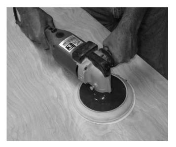
**Figure 8-4** Using a 7" electric orbital polisher with a foam disc sanding pad.
