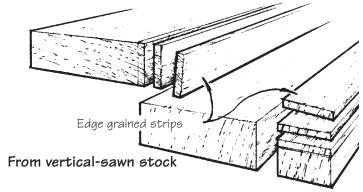
**Figure 9-1** Alternate methods for cutting your own vertical grain planks.
