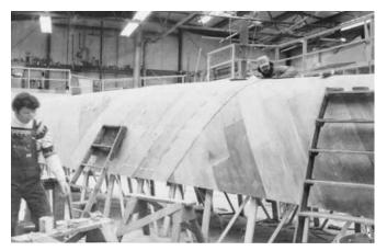
Figure 21-18 Installing a second layer of planking.
