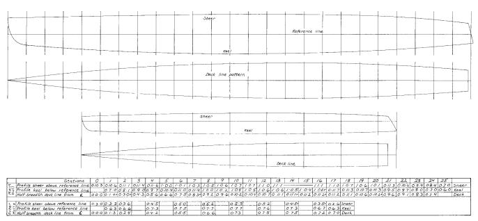
Figure 25-35 Hull and deck panels for Victor T, offsets given in feet, inches and eighths of an inch.
