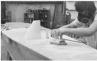
glossy or shiny and follow the directions given for fiberglass preparation. Test the product in an inconspicuous area to be sure that it will bond to epoxy. If any product fails to dry within the period specified on its packaging, try a different brand or use a primer.
