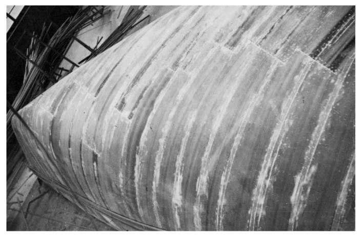
**Figure 21-3** Veneers in interlaminate layers of this laminated hull are butted randomly. This reduces scrap and eases lay up without sacrificing the strength of the hull. Note the final layer of veneer being laid fore and aft at the lower left.
