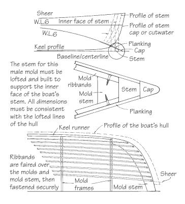
Figure 20-4 Lofting and set-up of a mold/stem assembly.
