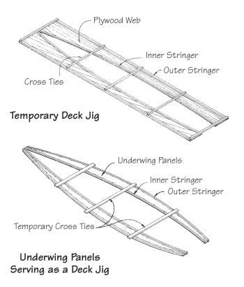
Figure 25-12 Typical deck jig and typical underwing panel.
