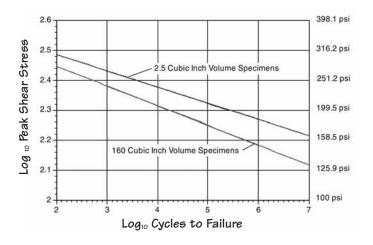
Figure C-16 Rolling Shear Fatigue Trends for Blade Laminate.
