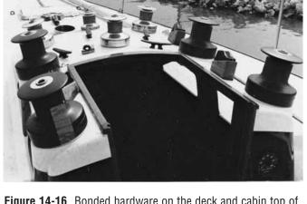
**Figure 14-16** Bonded hardware on the deck and cabin top of IOR  $\frac{1}{2}$ -ton racer *Hot Flash*. Several of the fittings have pads that were cast in place.
